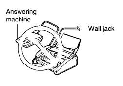
Do not connect an answering machine when using the TEL/FAX mode.
